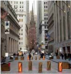
Image 4. NoGo barriers - security elements within the Wall Street zone. bronze sculptural forms integrated with lighting (A), seats integrated with pneumatically lowered crossing posts (B).
