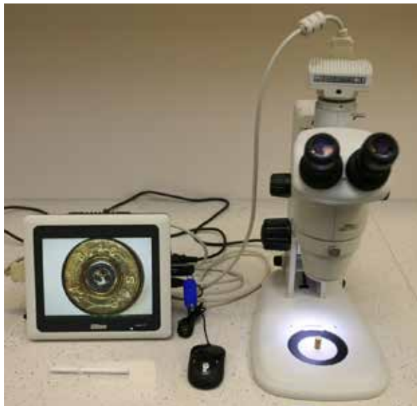
Fig. 1. The stereomicroscope integrated with microscopic digital camera and LCD screen.
