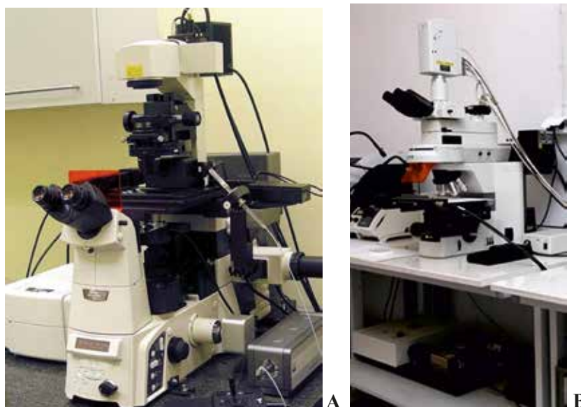
Fig. 3. Inverted confocal microscope Nikon TiE Eclipse A1 with microselection and laser microdissection (A) optical microscope with the C1 confocal equipment Nikon Eclipse 80i (B).
