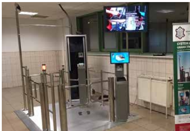
Pic. 2. Test biometric gate developed by Military University of Technology.
